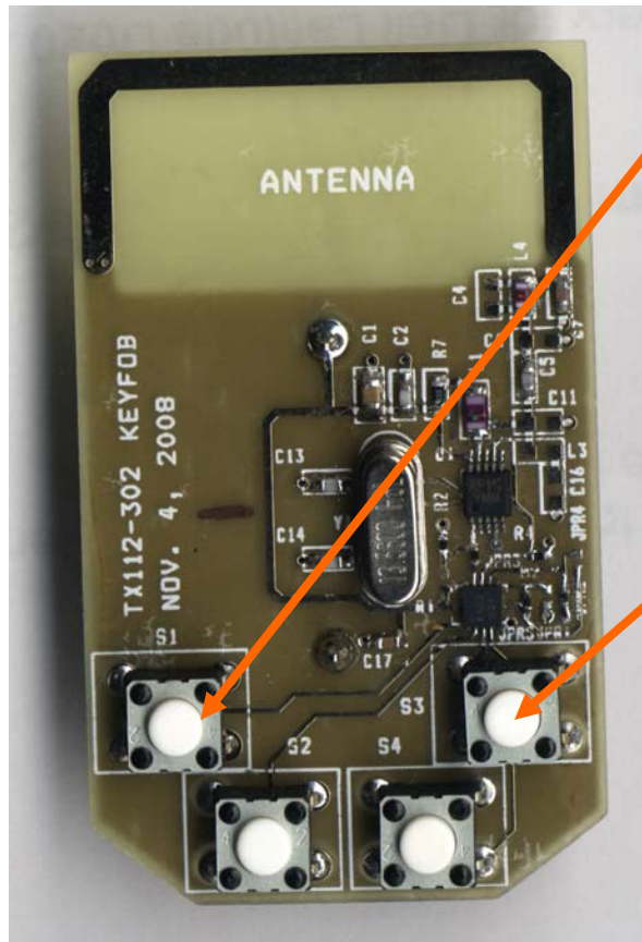
MICRF302 + MICRF112 KeyFob Reference Design
